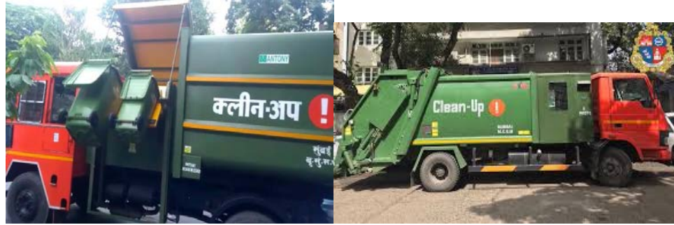
Side Loading Compactor- introduced for first time in India by MCGM
